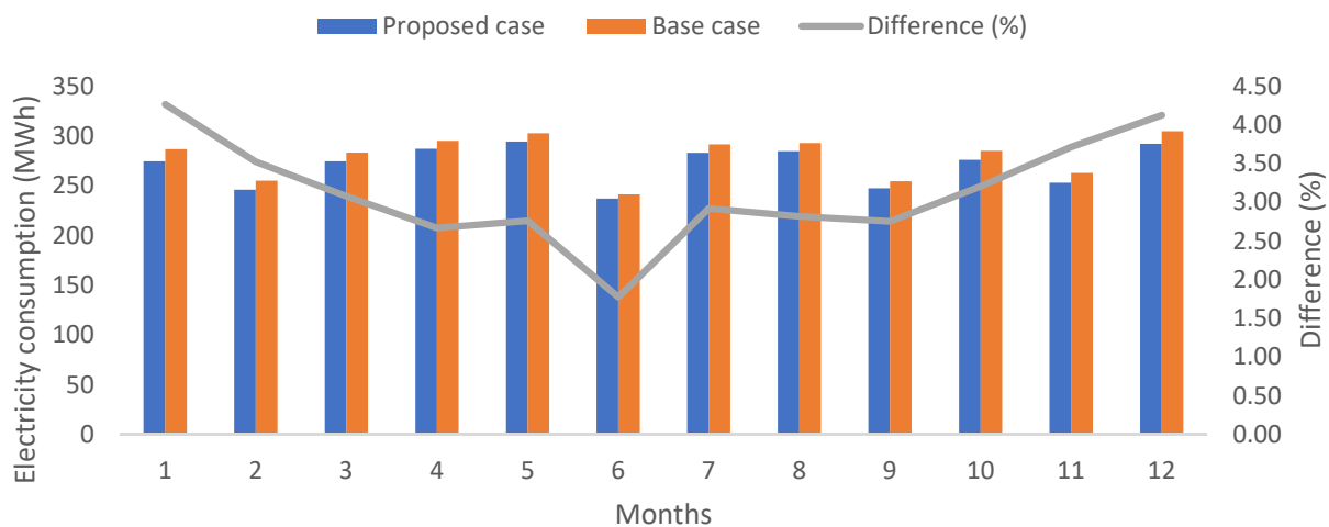
Figure 14. Comparison of monthly electricity consumption for cooling (only for occupied hours). Own elaboration.
