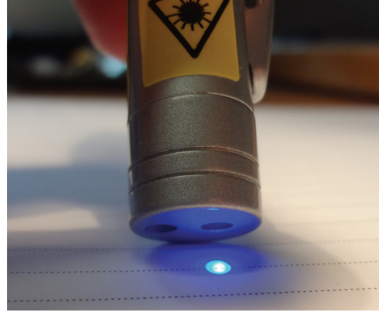
FIGURE 2: Violet laser stimulation with very low output power ( 1 \text{ mW} ). The beam area was about 0.5 \text{ cm}^2 , resulting in a power density of about 2 \text{ mW}/\text{cm}^2 [8].
