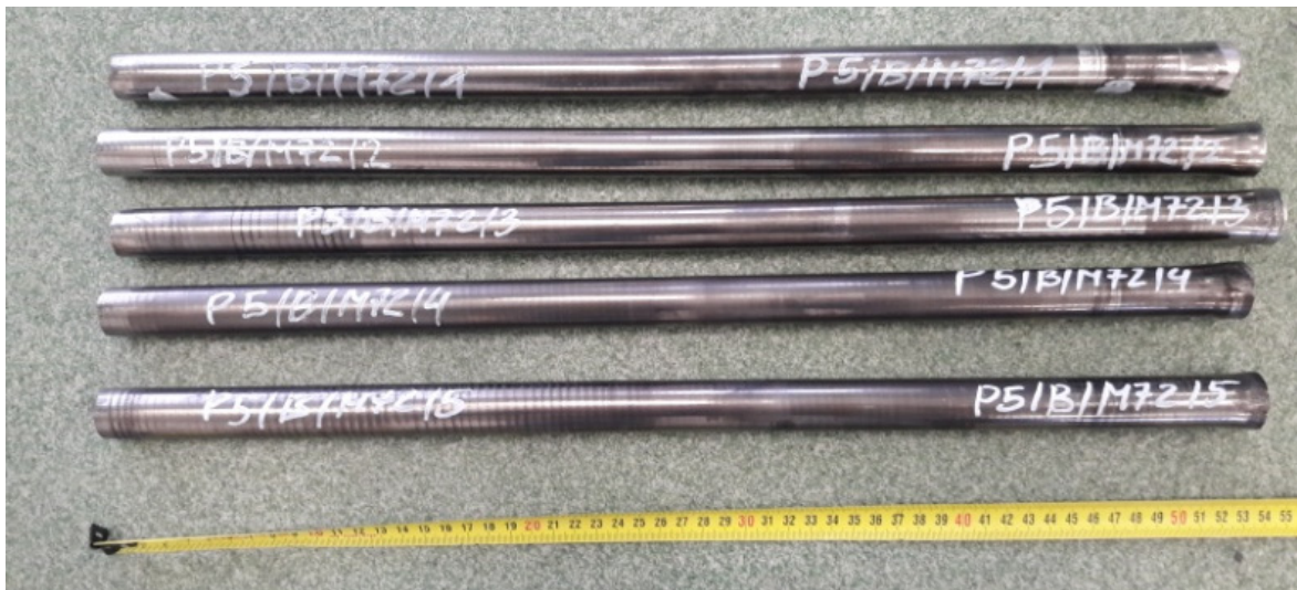
Figure 5. View of rods samples (WHA) after cold swaging.
