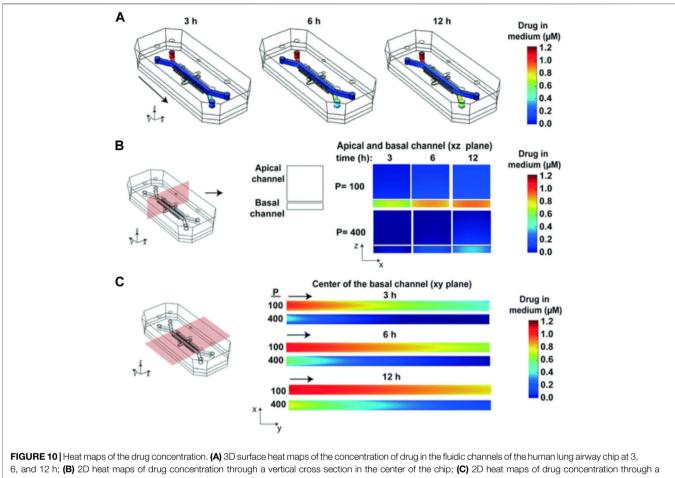
horizontal cross section in the center of the basal channel (Grant et al., 2021).
