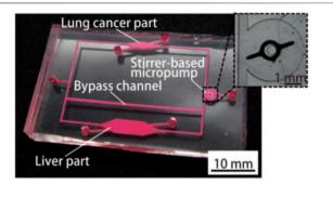
**FIGURE 8** | Photograph of the fabricated organs-on-chips with a liver part, a lung cancer part, and other parts connected by micro-channels (Shinha et al., 2020).
