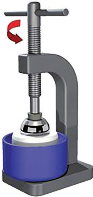
**Fig. 1** Vice clamp to assemble metal head in polyethylene outer head (picture courtesy of LIMA Corporate, Italy).
