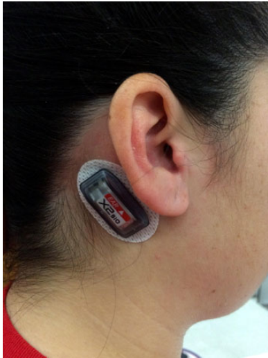
Figure 1. The xPatch sensor adhered over the right mastoid process.
