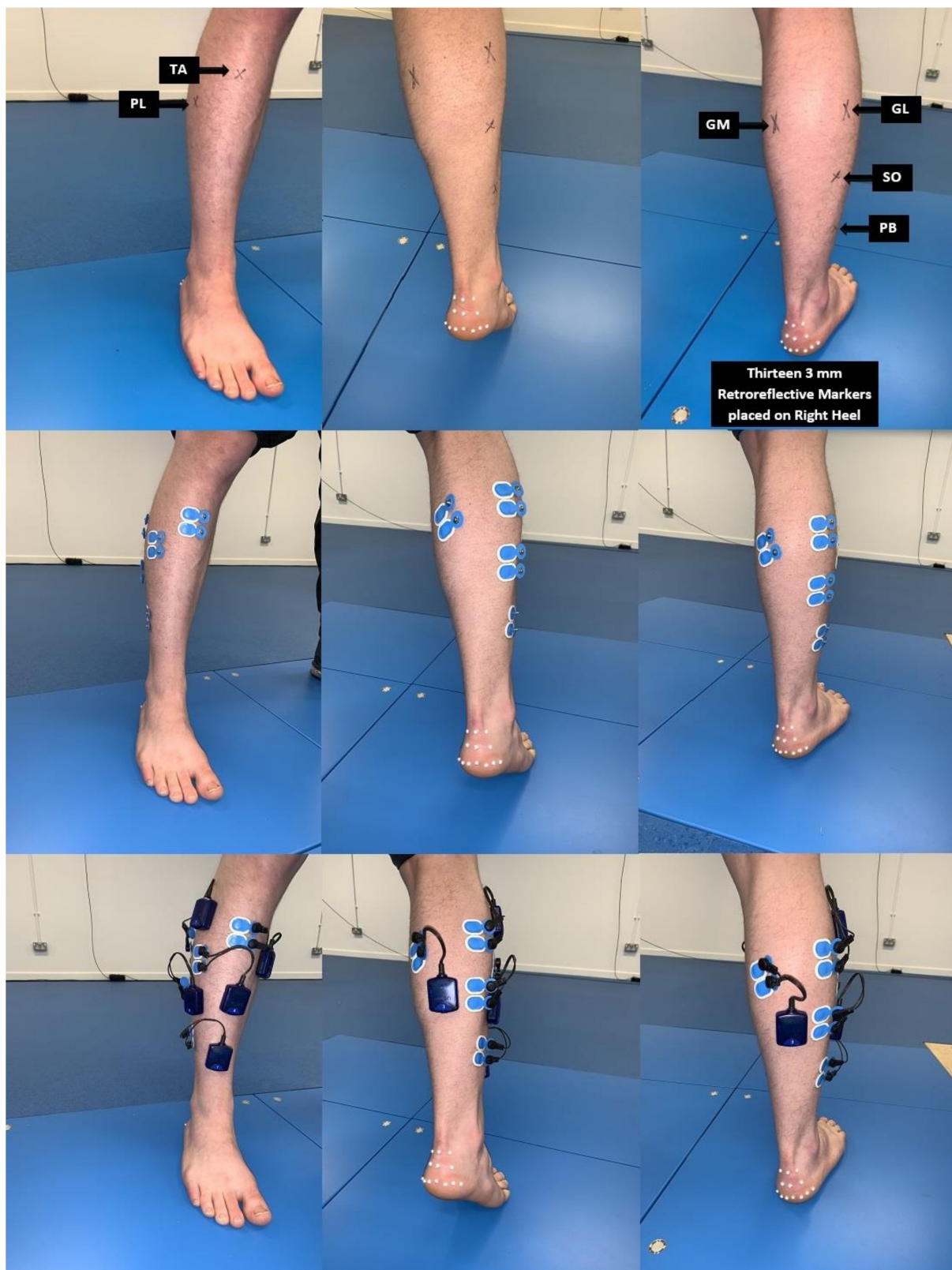
Figure 2. Row 1: Presented on the right leg are marked positions of the lower limb muscles. Row 2: The marked positions are covered with self-adhesive AMBU surface electrodes positioned on the GM, GL, SO, TA, PL and PB. Row 3: The self-adhesive AMBU surface electrodes were connected to the Myon 320 transmitters (transmitters were secured to the calf muscles with double-sided tape). The columns represent the baseline, unloading (concentric) and loading (eccentric) phases of the heel raise task, respectively. Retroreflective markers on the heel were used for tracking the heel phase positions.
