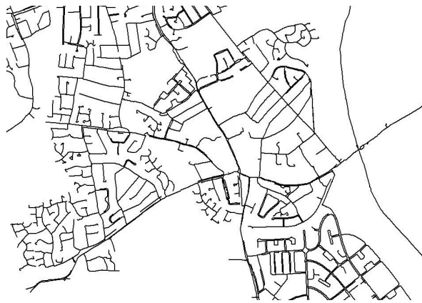
Figure 1. An example water supply pipe map for a region in the UK. The range of pipe layouts can be seen: straight pipes, curved pipes, and pipes with sharp corners. The scale of the map is 2 km from the bottom to the top.
