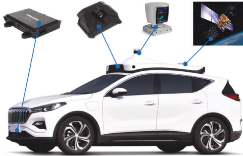
FIGURE 1: structure of the intelligent vehicle environment sensing system.
