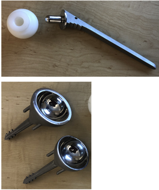
Figure 1. Pictures showing the femoral component with its smooth taperless trunnion allowing the all-polyethylene head to freely rotate. The acetabular components shown were available in thick- and thin-walled versions. Both versions had the same central long spike with 3 smaller spikes around the center spike.
