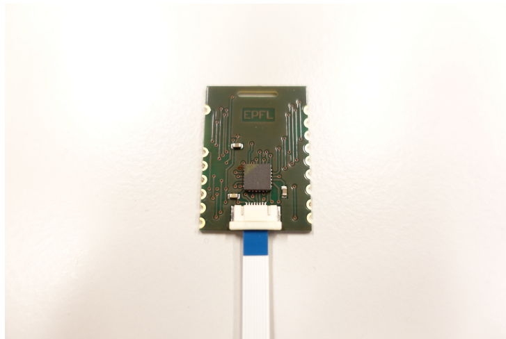
Figure 9. PCB with ANTIGONE packaged chip.
