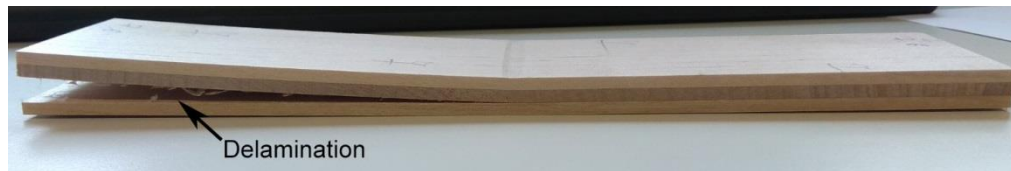
Figure 3. Delamination in the low-density polyethylene (LDPE)-bonded plywood samples during the determination of bending strength.
