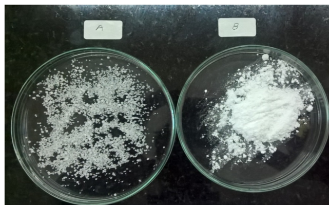
Fig. 3. A: Commercial Pentaerythritol B: Ground Pentaerythritol powder of < 100-micron size.
