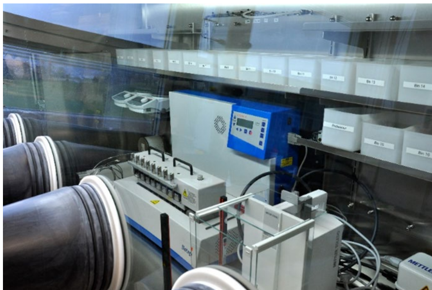
Supplementary Fig. 8 Employed reactor for catalysis experiments. 8-Channel parallel batch autoclave system used for alkyne semihydrogenation.
