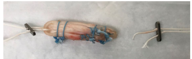
Figure 5. Button loop rupture from load-to-failure test.
