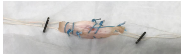
Figure 4. Suture-tendon rupture from load-to-failure test.
