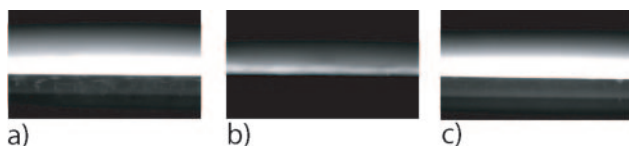
Figure 5. Comparison of hybridization images: images of sections of the Cy3-hybridized capillary edge (a–c). The central region (b) consists of synthesized target DNA containing a single mismatch whereas the flanking regions (a,c) consist of target perfect match sequences.
