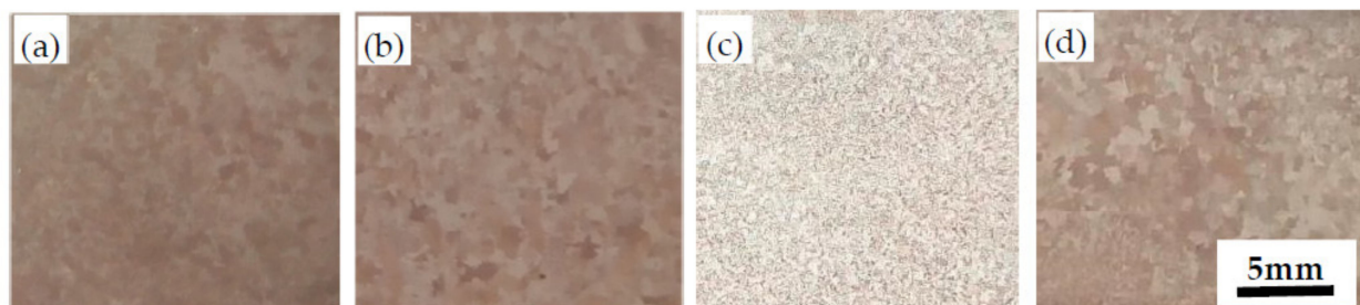
Figure 4. Macrostructure of the ZCuPb20Sn5Ni3-0.1P-yB alloy. (a) B = 0.0 wt.%; (b) B = 0.05 wt.%; (c) B = 0.1 wt.%; (d) B = 0.2 wt.%.
