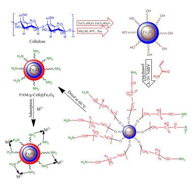
**Figure 1.** Proposed scheme for synthesis and functioning of poly(acrylamide)-g-Cell@Fe<sub>3</sub>O<sub>4</sub> (PAC@Fe<sub>3</sub>O<sub>4</sub>) nanocomposites.
