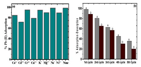
**Figure 11.** (a) Effect of other competitive ions on the adsorption of Pb(II) by PAC@Fe<sub>3</sub>O<sub>4</sub>. (b) Adsorption–desorption plot for Pb(II) on PAC@Fe<sub>3</sub>O<sub>4</sub>.
