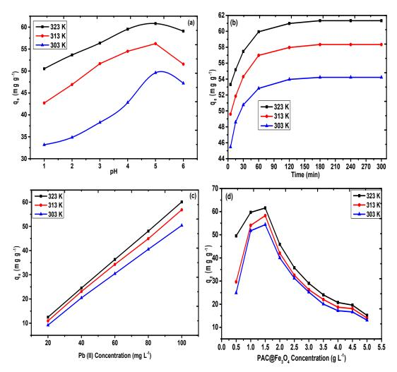
**Figure 8.** Effect of (a) pH, (b) agitation time, (c) Pb(II) concentration, and (d) adsorbent dose on adsorption of Pb(II) on PAC@Fe<sub>3</sub>O<sub>4</sub>.
