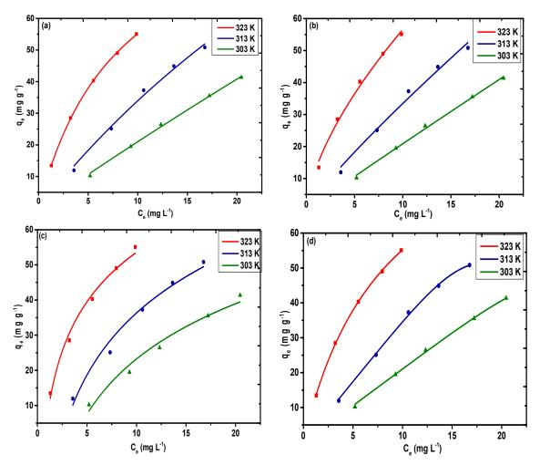
**Figure 9.** Adsorption isotherms for (a) Langmuir, (b) Freundlich, (c) Temkin, and (d) Redlich–Peterson models for Pb(II) on PAC@Fe<sub>3</sub>O<sub>4</sub> at 323, 313, and 303 K (dose =  $1.5 \text{ g L}^{-1}$  and pH 5).
