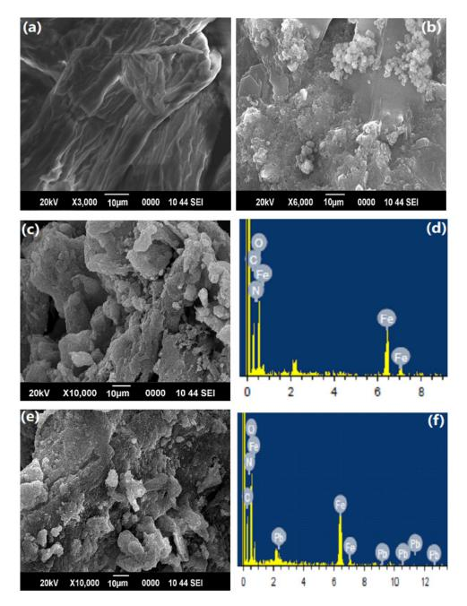
**Figure 3.** SEM images of: (a) cellulose; (b) PAM; (c,d) PAC@Fe<sub>3</sub>O<sub>4</sub> and its EDX image before adsorption; and (e,f) PAC@Fe<sub>3</sub>O<sub>4</sub> and its EDX image after adsorption of Pb(II).
