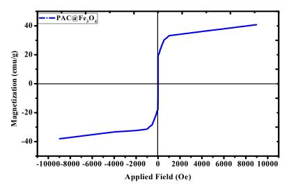
**Figure 7.** Magnetization curve for the PAC@Fe<sub>3</sub>O<sub>4</sub> nanocomposite at room temperature.
