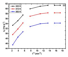
**Figure 10.** Non-linear regression plot of the (a) pseudo-first-order model, (b) pseudo-second-order model, and (c) intra-particle diffusion plot for Pb(II) on PAC@Fe $_3$ O $_4$  at 323, 313, and 303 K (dose = 0.03 g and pH 5).
