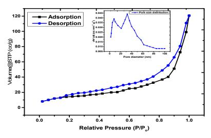
**Figure 6.** N<sub>2</sub> adsorption–desorption curve and BJH pore size distribution for the PAC@Fe<sub>3</sub>O<sub>4</sub> nanocomposite.
