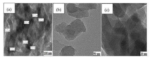
**Figure 4.** TEM images of PAC@Fe<sub>3</sub>O<sub>4</sub> showing nanoparticle dispersion in the polymer matrix at (a) 100 nm, (b) 50 nm, and (c) 20 nm magnification ranges.
