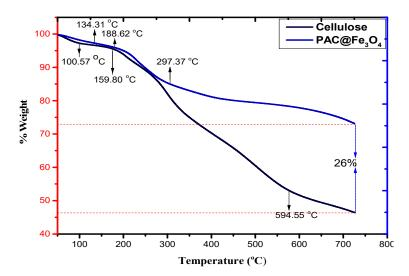
Figure 5. TGA spectra of cellulose and PAC@Fe<sub>3</sub>O<sub>4</sub> in a temperature range of 0–800 °C.
