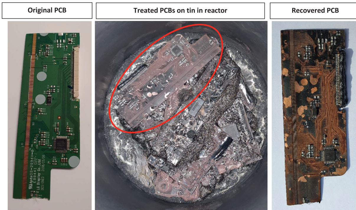
Fig. 9. Results of pyrolysis of PCBs on molten tin. Left: original PCB, middle: the situation after opening the cooled down reactor (circle shows the PCB on the right), right: recovered PCB.
