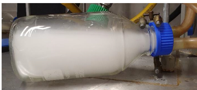
Fig. 5. Photo of the interceptor vessel during one of the experiments on aluminium-laminated plastics.
