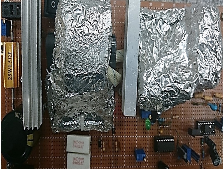
Figure 2. The prototype of constructed high voltage power supply module.
