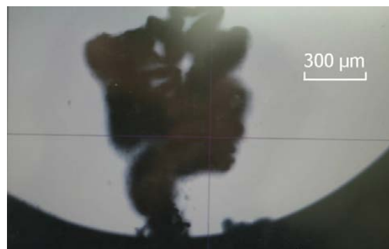
Figure 9. Continuous and ribbon-like chip.
