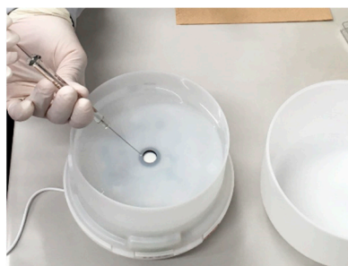
Figure 2. Preparation of diffusing and collecting test: Dropwise 0.5 mL of essential oils and effective component to 350 mL water in the aroma diffuser.
