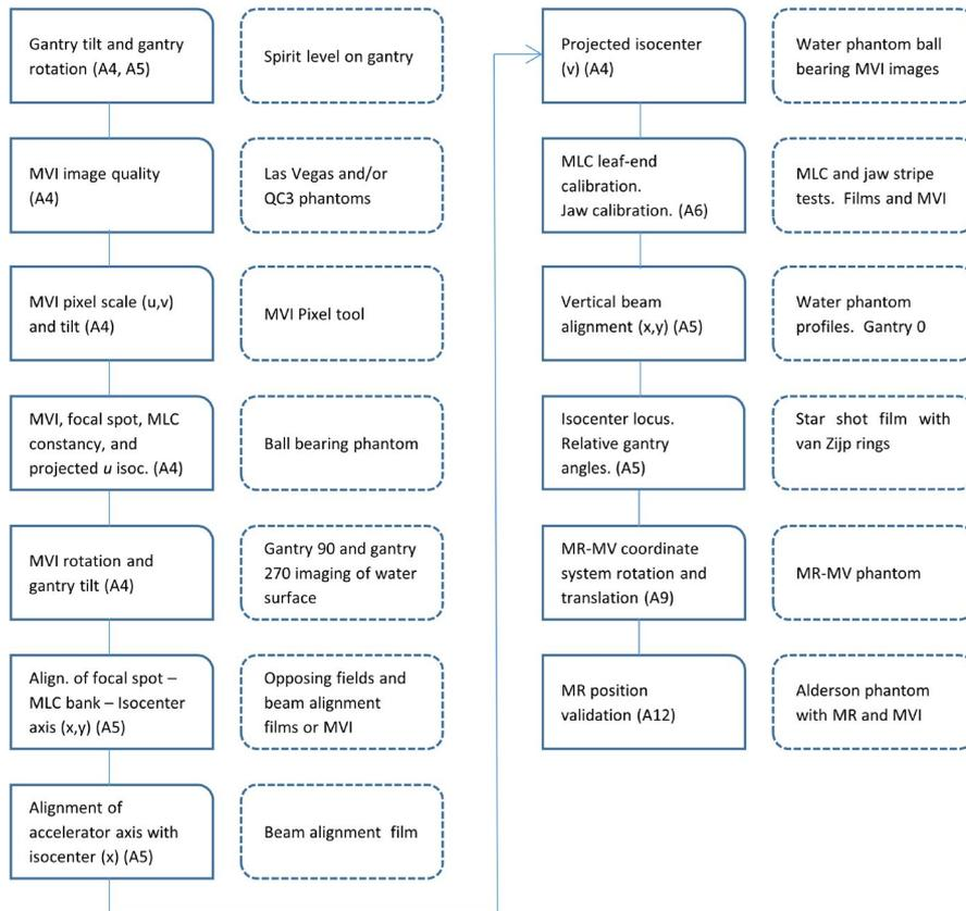
**FIG. 2** Schematic of independent system alignment checks for the linac component of the MRI-linac
