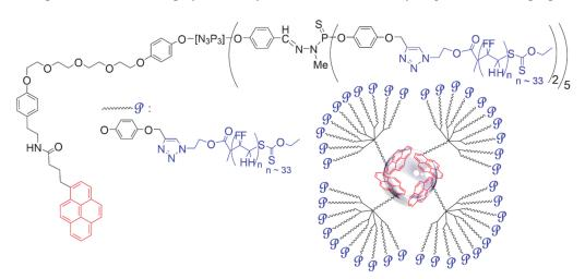
**Figure 4.** Chemical structure of a dendron bearing vinylidene fluoride polymers on the surface, and used for coating cobalt nanoparticles covered by graphene.
