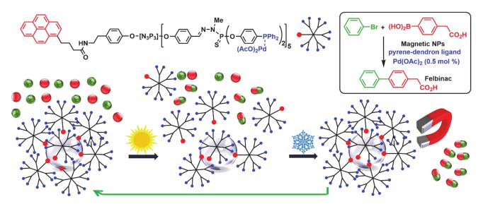
**Scheme 12.** Non-covalent grafting of catalytic dendrons onto cobalt nanoparticles covered by graphene layers, and their use as catalysts in Suzuki couplings. Example of coupling for the synthesis of Felbinac. Recovering and re-use were carried out eleven times, with a quantitative yield in Felbinac in all cases.
