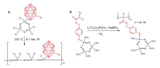
**Scheme 3.** Examples of polymerization reaction of  $AB_5$  derivatives of cyclotriphosphazene. (**A**) Polymerization of  $N_3P_3$ . (**B**) Polymerization of a substituent of  $N_3P_3$ .
