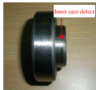
Figure 13. Bearing inner race defect.
