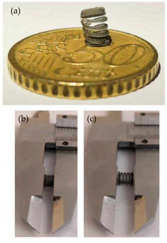
Figure 7. SL printed micrometric spring. (a) Geometry details, (b) compression, (c) release.
