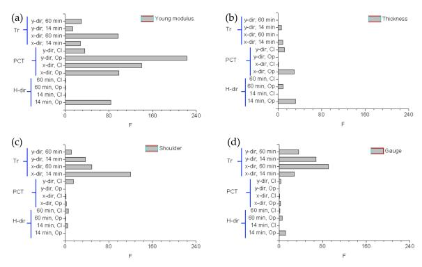
**Figure 6.** ANOVA: plot of the F values computed for **(a)** Young's modulus, **(b)** thickness, **(c)** shoulder width, **(d)** gauge width.
