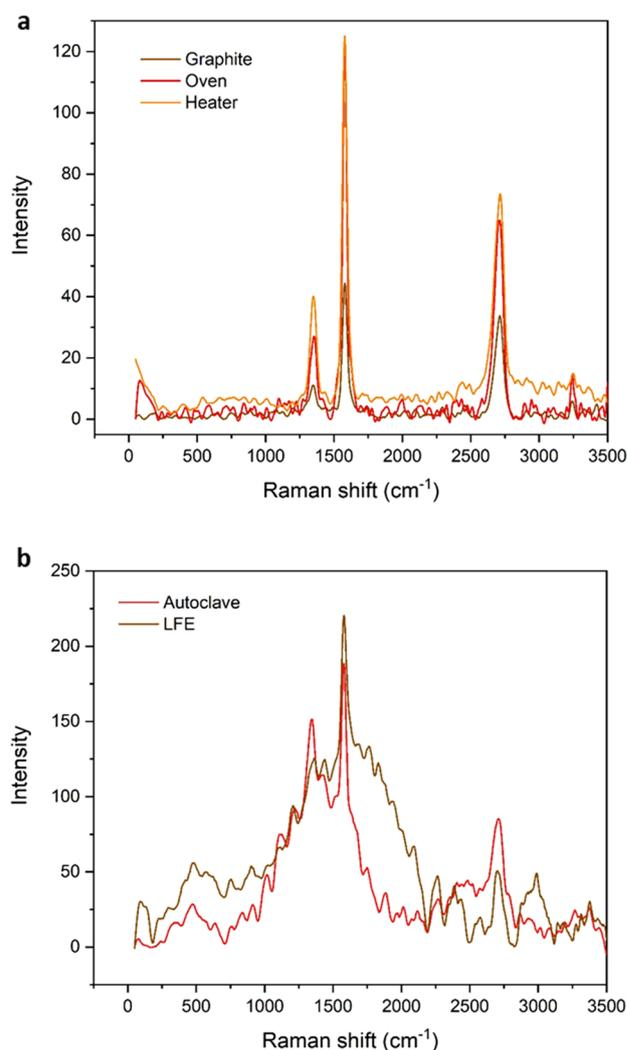
**Figure 6.** Vibrational modes of FGPs samples in Raman spectra. **(a)** Raman spectra of Graphite, Oven-, and Heater-method. **(b)** Raman spectra of Autoclave- and LFE-method.
