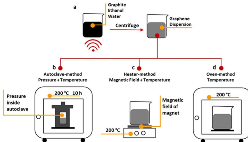
**Figure 1.** Dispersion of graphene and three different methods for investigating the effect of temperature, pressure, and magnetic field on the magnetization of graphene. (a) Dispersion of graphene dispersion by the liquid-phase exfoliation method. (b) Applying temperature and pressure by the Autoclave-method. (c) Applying magnetic field and temperature by the Heater-method. (d) Applying temperature by the Oven-method.
