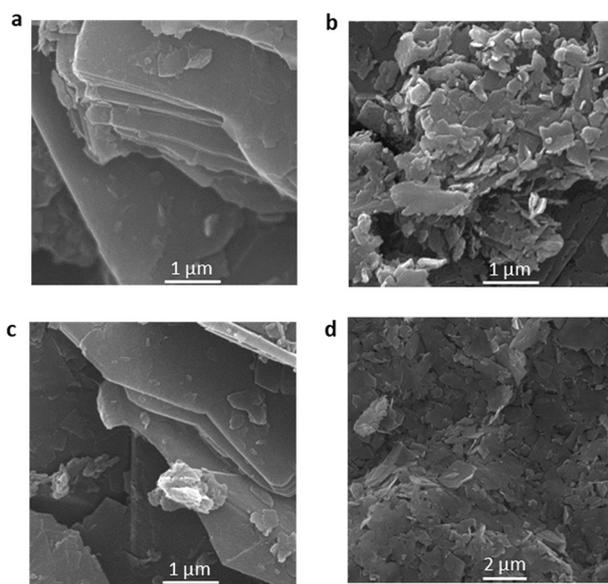
**Figure 5.** SEM images of FGPs. (a–d) the Oven, Autoclave, Heater, and LFE, respectively. The difference between stacking and aggregation process is obvious in the images. (a,c) Stacking. (b,d) Aggregation.
