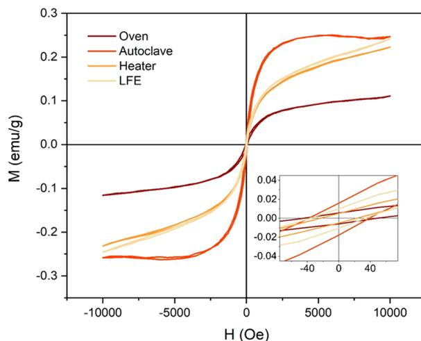
**Figure 2.** VSM diagram of FGPs to determine the contribution of temperature, pressure, and magnetic field in magnetism. The hysteresis loop of all samples and the zoom part of diagram  $-90 < H < 90$  (Oe) and  $-0.045 < M < 0.045$  (emu/g) in the inset.
