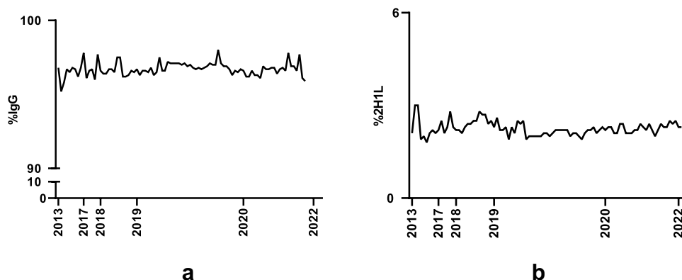
Fig. 2 Purity and impurity levels in SB5 batches analyzed by non-reduced capillary electrophoresis-sodium dodecyl sulfate (CE-SDS). a Purity levels of IgG and b impurity levels of 2H1L
