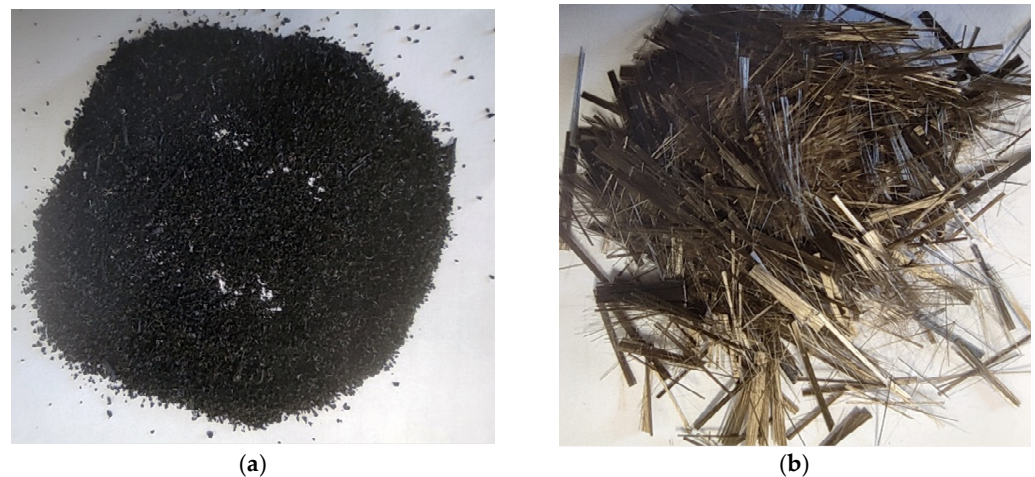
Figure 1. Physical appearance of the materials used. Powdered rubber (a) and carbon fibers (b).
