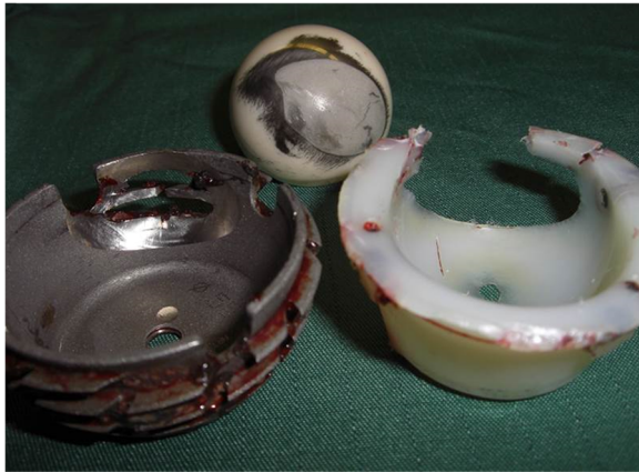
Fig. 6 Intraoperative picture showing totally worn-out liner and affected cup
