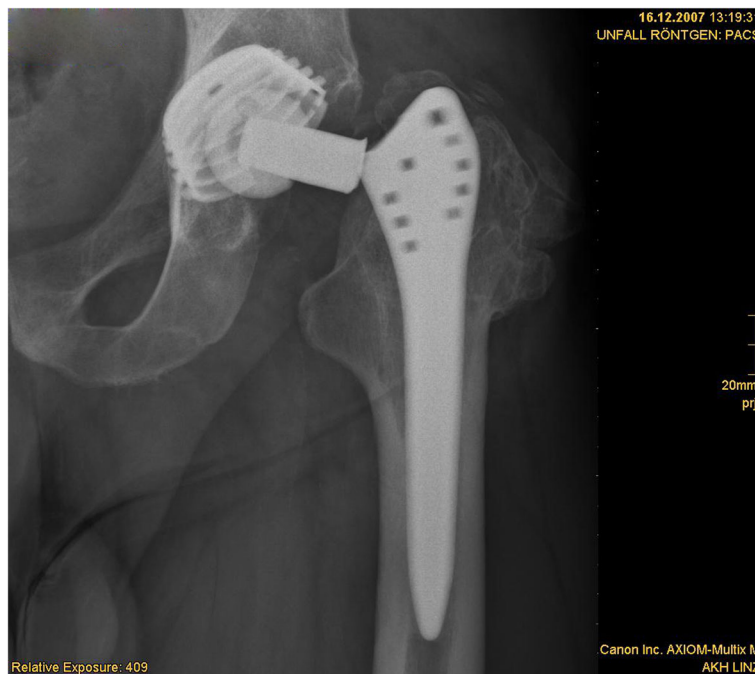
Fig. 7 Radiograph showing implant fracture after 20 years
