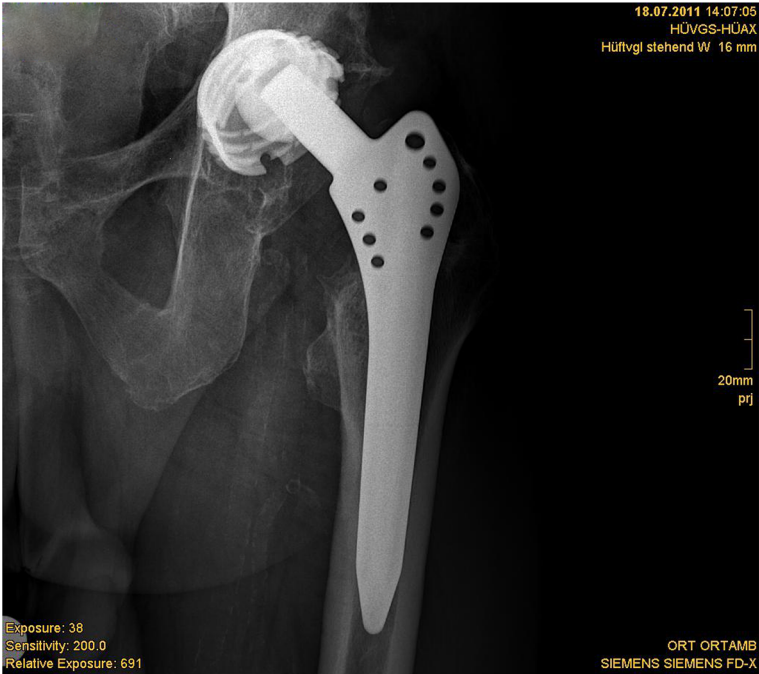
Fig. 5 Radiograph showing totally worn-out liner after 25 years
