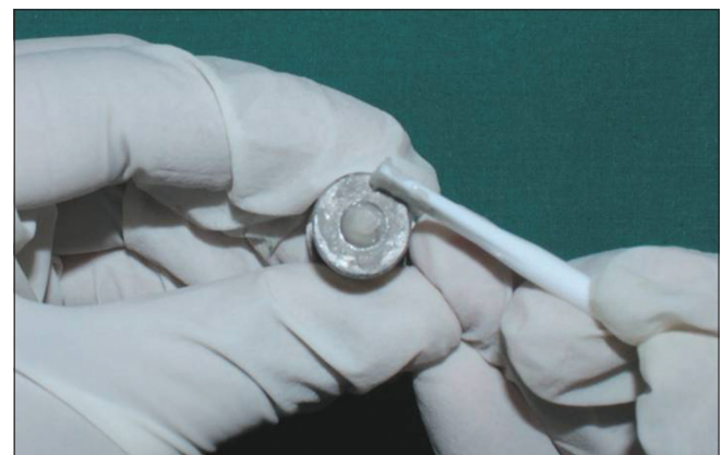
Figure 3: Packing of the composite core build-up material in the lower mold space
