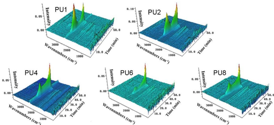
Figure 7. The 3D surface graphs of the FTIR spectra of the evolved gases produced by PUFs.
