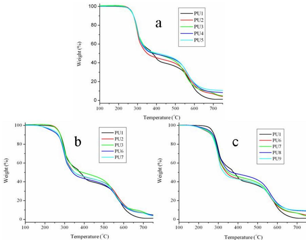
**Figure 6.** The thermal stabilities of PUFs (a) the effects of EG/APP on the thermal stability of PUF, (b) the effects of micro-PCMs on the thermal stability of PUF/EG composite, (c) the effects of EG/APP on the thermal stability of PUF/micro-PCMs composite.
