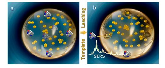
**Figure 9.** Schematic of the one-pot controlled synthesis of AuNPs@MIPs for improved SERS sensing (**a**) [89]. After the template removal, target molecules can selectively rebind with the cavities, and the analytes can closely contact with the Au NPs in the imprinted layer (**b**), which significantly improves the selectivity and sensitivity.
