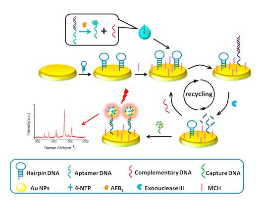
Figure 7. A recycling SERS-based aptasensor chip using the exonuclease to amplify the Raman signal [73].
