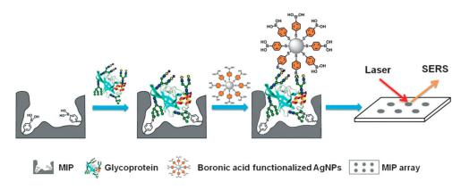
**Figure 11.** Schematic representation of the boronate-affinity sandwich assay of glycoproteins [122]. Target glycoprotein can be captured specifically by a boronate-affinity MIP array. The captured glycoprotein is then labeled with boronate functionalized AgNPs for SERS detection.
