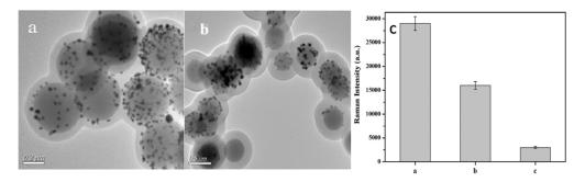
**Figure 10.** The TEM images of  $SiO_2/Ag/MIPs$  with different shell thickness: 40 nm (**a**), 170 nm (**b**) and (**c**) the SERS detections of different thicknesses of  $SiO_2/Ag/MIPs$  to the same concentration of R6G at  $10^{-6}$  mol L<sup>-1</sup> (40 nm (**a**), 100 nm (**b**), 170 nm (**c**)) [106].
