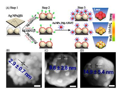
**Figure 6.** (A) A polyadenine mediated core-satellite nanoassembly immobilized on the silicon wafer [66]. (**B**–**D**) are SEM images of the interparticle gaps of satellite Au NPs of Au-Au NPs mediated by Poly A10, Poly A30, and Poly A50.
