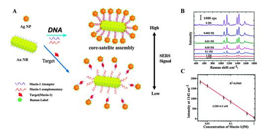
**Figure 8.** (**A**) Mucin-1 detection based on SERS with bimetallic core (gold nanorods)—satellite (silver nanoparticles) assemblies [77]. (**B**) SERS spectra of Mucin-1 detection; (**C**) Standard curve for Mucin-1 detection with corresponding peak intensities at 1142 cm<sup>-1</sup>.
