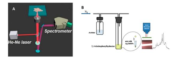
Scheme 1. (A) Schematic diagram of Raman detection; (B) Schematic diagram of chemical reaction assisted SERS detection [17].
