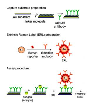
Figure 4. SERS-based immunoassay platform [35]. Antibodies were fixed on a platform to capture antigen, Ag or Au NPs conjugated with both Raman tags and detection antibodies can then be captured for SERS detection.
