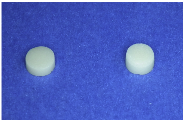
Fig. 1 Tested samples of the zirconia and the porcelain.
