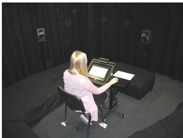
Figure 1. Experimental setup in AuraLab with five loudspeakers and additional porous floor absorbers.
