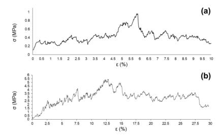
**Figure 4.** Stress–strain  $(\sigma - \varepsilon)$  curve of dolomite-foamed D-800 (a) and D-850 scaffolds (b).
