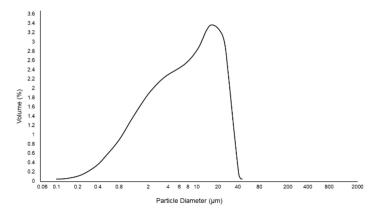
**Figure 1.** Particle size distribution of 47.5B glass powder (sieved below 32  $\mu$ m) used for scaffold manufacturing.
