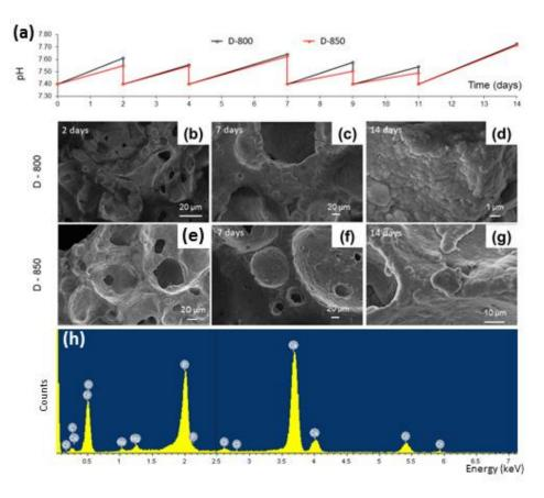
**Figure 5.** Bioactivity tests in simulated body fluid (SBF): pH variation as a function of the immersion time (a); FE-SEM micrographs of the surface of D-800 (**b**–**d**) and D-850 (**e**–**g**) scaffolds after immersion in SBF for 2, 7, and 14 days; example of EDS spectrum of the newly formed surface layer on D-850 sample after seven days in SBF (**h**).
