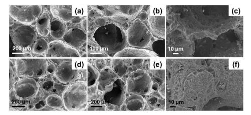
Figure 2. FE-SEM images of dolomite-foamed scaffolds D-800 (a-c) and D-850 (d-f) at different magnifications.
