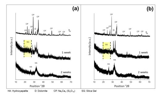
**Figure 6.** XRD patterns after immersion in SBF at different time points related to D-800 (a) and D-850 (b) scaffolds. CP = crystalline phase ( $Na_4Ca_4(Si_6O_{18})$ ) of sintered glass-ceramic scaffold; D = residual dolomite; SG = halo associated to the silica gel layer; HA = hydroxyapatite.
