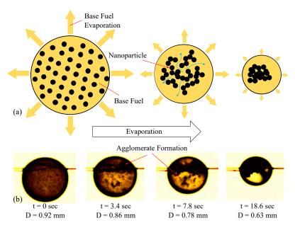
**Figure 5.** (a) Proposed mechanism of base fuel diffusion suppression by coagulation of nanoparticles; (b) time lapse of agglomerate formation in a droplet of 0.25% MWNT in jet fuel.
