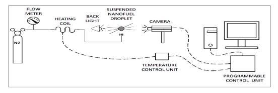
Figure 2. Schematic of droplet evaporation arrangement.
