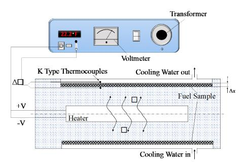
Figure 1. Schematic of thermal conductivity measurement device.
