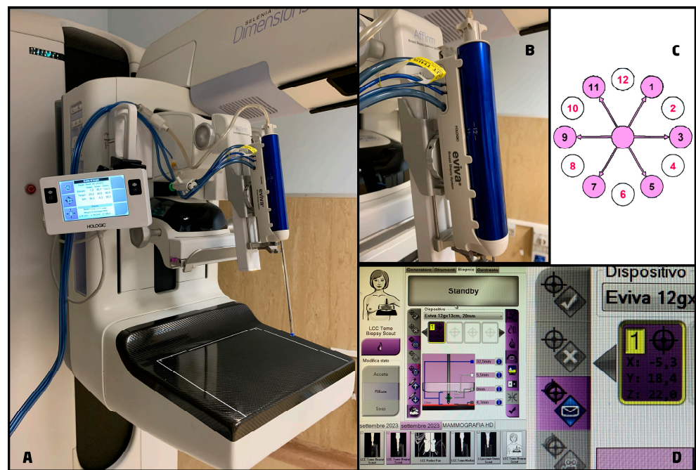
Figure 2. Biopsy system. (A) Affirm ® Upright Breast Biopsy Guidance System (Hologic, Bedford, MA, USA), it added to the mammography unit to perform 2D or DBT-guided biopsies and it is equipped with a monitor to display the biopsy coordinates and the needle position; (B) Eviva ® breast biopsy system (Hologic, Bedford, MA, USA), it is available with different needles options and makes possible saline lavage and constant aspiration thanks to its connection to the vacuum console; (C) scheme showing the range of movements of the biopsy system for tissue sampling at even (white circles) and odds (pink circles) positions; (D) an example of how to calculate the coordinate for the biopsy using a 12 gauge needle.
