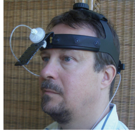
FIGURE 1: Measurement setup of nasal pressure signal with nasopharyngeal catheter.
