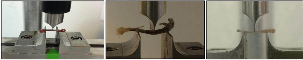
Fig. 1. Femur (left), Tibia (middle) and Ulna (right) loaded in three point bending test.
