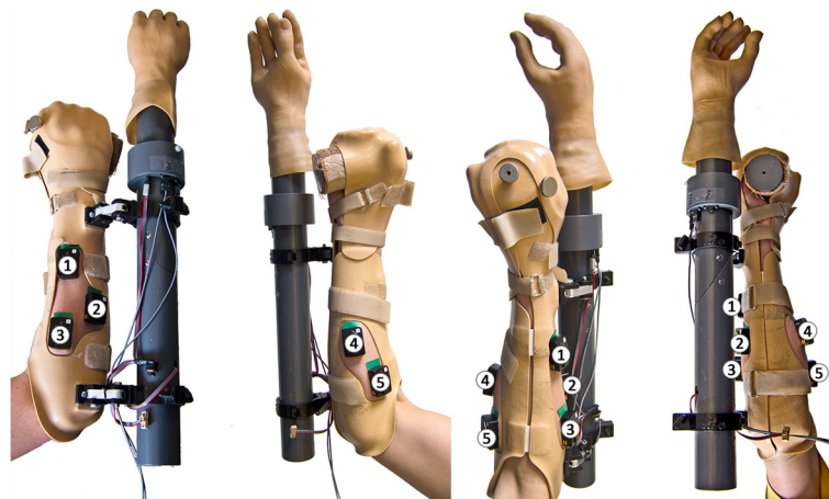
Figure 1 Socket design and electrode placements demonstrated on one of the subjects (lateral, medial, top and bottom view, respectively).
