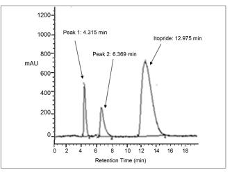
Fig. 1: LC-PDA chromatogram of itopride along with degradation products
