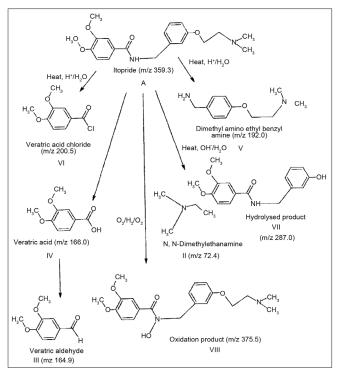
Fig. 3: Proposed degradation route of itopride Proposed degradation route followed by itopride leading to the formation of degradation products II-VIII
