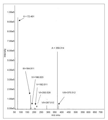
Fig. 2: LC-MS spectrum of itopride and its degradation products II-VIII. The label A denotes itopride
