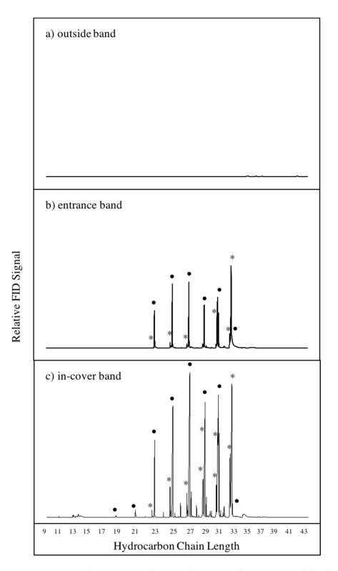
**Figure 2.** Representative gas chromatograms of compounds extracted from (**a**) an outside band, (**b**) an entrance band, and (**c**) an in-cover band. Alkanes indicated with dots (•) and alkenes indicated with asterisks (\*). All bands were deployed in the same hive at Awbury Arboretum on 07/15/2016.
