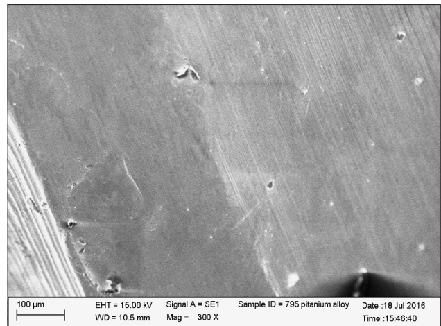
Figure 2: SEM image of laser-etched abutment
