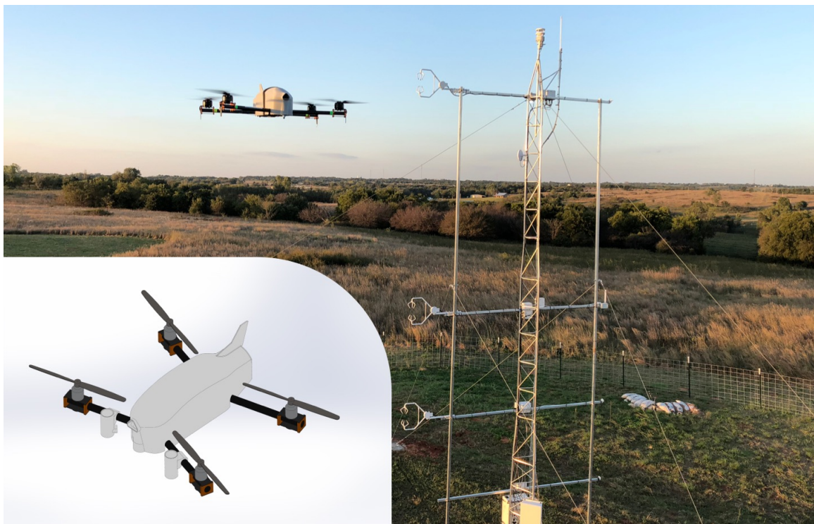
Figure 1. Photograph of the OU CopterSonde rwUAS (Norman, OK, USA) in flight next to an experimental 10 m flux tower, and a 3D model (inset) of the aircraft in flight. The 3D model design is the one used in this study, which includes sensors located in solar shields underneath the front two propellers and housed in a ducted fan on the front of the main body. The solar shields and main body with the ducted fan were 3D printed in white and grey plastic, respectively.
