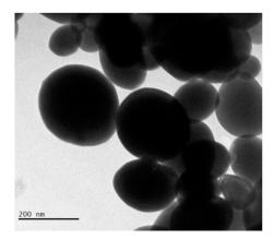
**Figure 3.** Transmission electronic microscopic capture of bismuth oxide nanoparticles with average diameter ranging from 150 nm to 200 nm. Picture is reprinted with permission from Abudayyak et al. [57].
