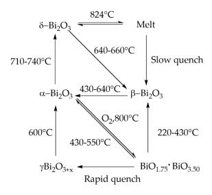
Figure 2. Scheme of phase transition of bismuth oxide.
