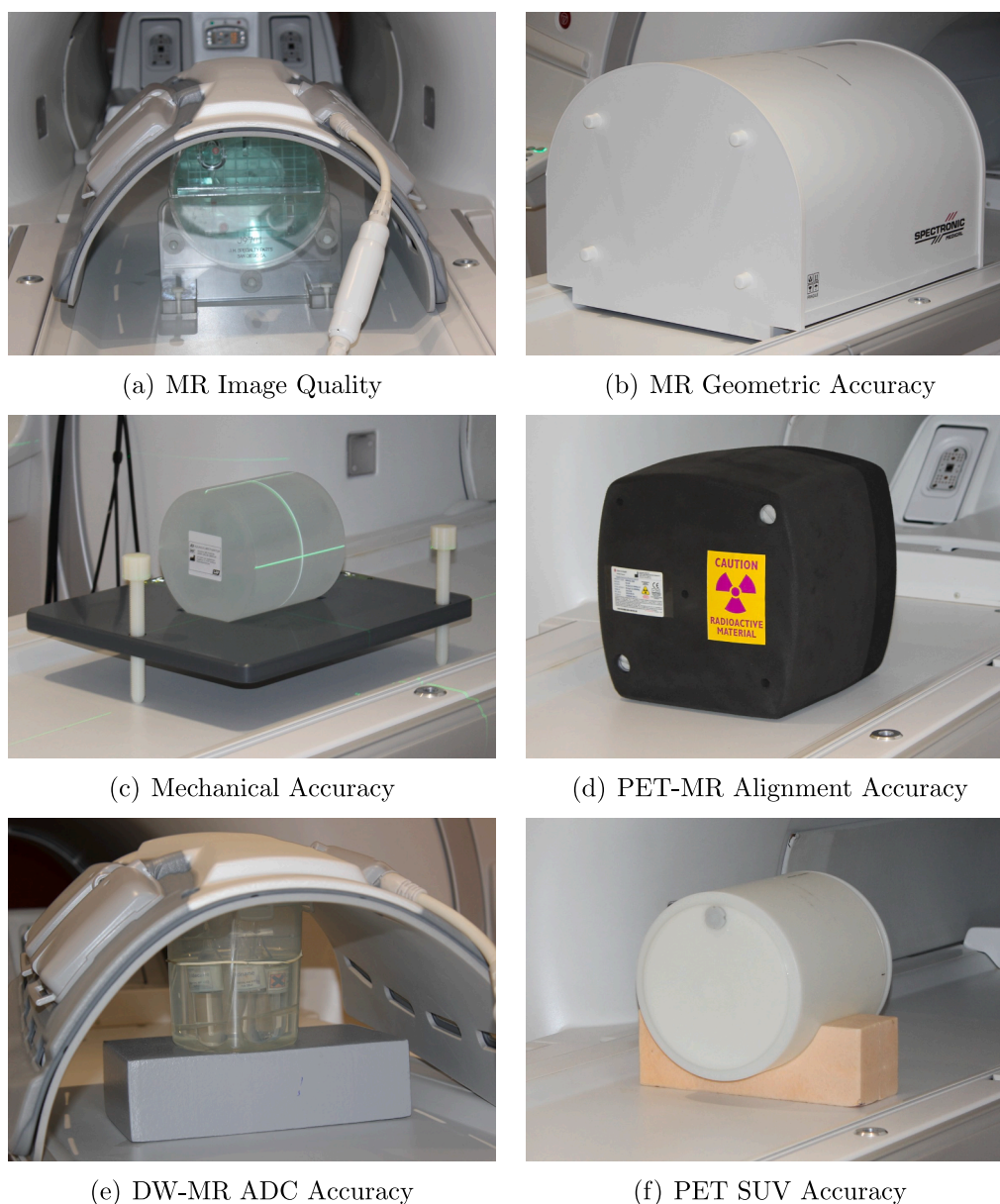
Fig. 1. Photographs of the phantoms and setup used for each of the six QA tests evaluated. Each test was carried out three times on the same day using independent phantom setups (repeatability measurements) and once a month for 12 months (stability measurements). Images were acquired using the spine coil and anterior array coil for MR image quality and DW-MR ADC accuracy tests, and the in-built body coil/PET detector for the other tests.
