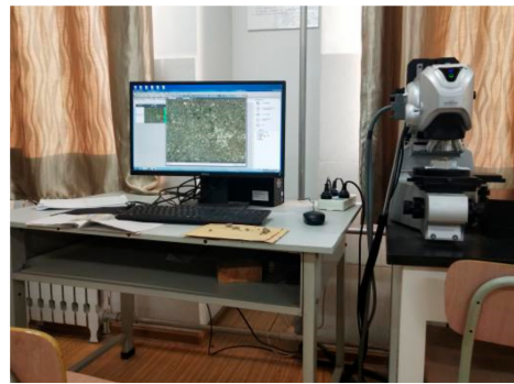
Figure 4. VK-X150 Laser 3D microscope.
