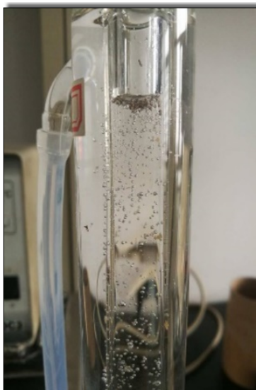
Figure 5. Apparatus setup for sand suspension ability test.
