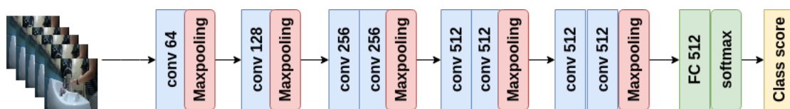
Figure 11. Coarse wall classifier: Model with RGB only.
